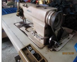
External photo(s) of the production unit(s) NC PA 7-17 Sewing Machine not Installed with Pulley Guard.JPG
